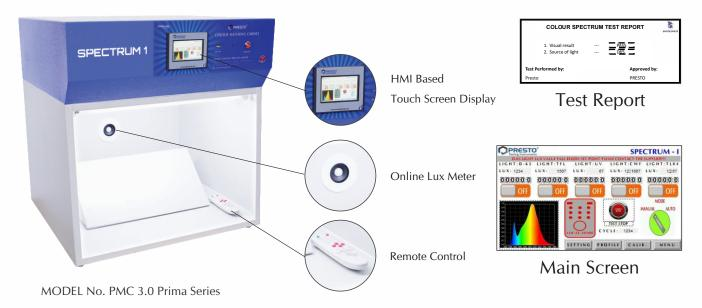
**Presto color matching cabinet Spectrum -1** is a simulation tool, which is mainly used in quality control. The color matching cabinet accurately corrects light types and thus allows direct comparison of products that must have special color characteristics. The color matching cabinet supports five possible lighting types. These colors are supplied as standard: ,"D65", "TL84, "UV", "CWF" and "TFL
